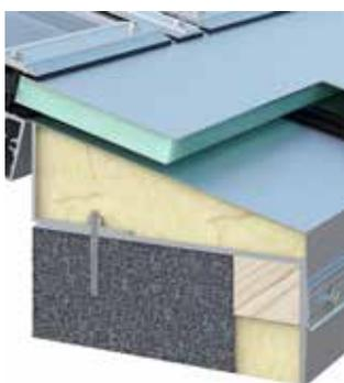
Installation on concrete upstand
