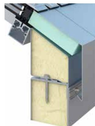
Installation on steel sheet upstand
