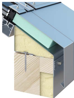
Installation on wood upstand
