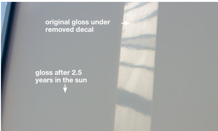
Realtime RV sidewall application with removed decals – 2.5 years
